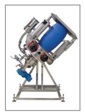
The DCS Inverter is ideal for emptying lumpy and agglomerated products requiring a contained environment, eliminating the need for downflow booths.
